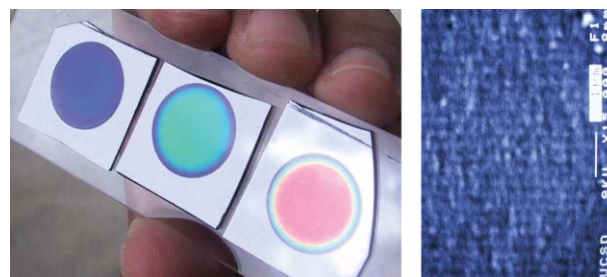
Fig. 3 Porous Si photonic crystals as inorganic analogues of the beetle shell. Left: Photograph of three one-dimensional photonic crystals made from porous Si. Right: Electron micrograph image showing the layered porous structure in a film. These samples are rugated structures, prepared by application of a sinusoidal current during etching. The different colors are produced using sine waves of different frequencies.
